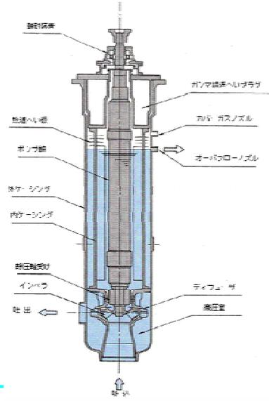
Intake pressure should be positive in order to prevent cavitation.
