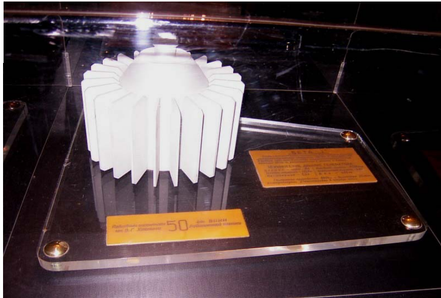
^{90}\text{Sr} Battery (KRI) 23,000Ci ^{90}\text{Sr} 150W
