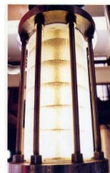
Figure 4. Section of the 10cm diameter single pulsed column at Sellafield showing the stainless steel mesh plates and a dispersion of aqueous drops in a continuous organic phase
