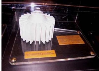
^{90}\text{Sr} Battery (KRI) 23,000Ci ^{90}\text{Sr} 150W
